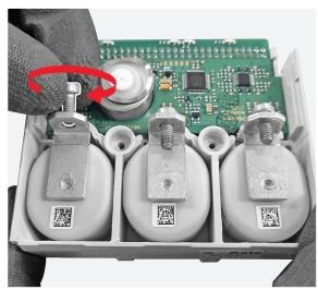
**53**Manually remove the wave spring located over the trip coil.
