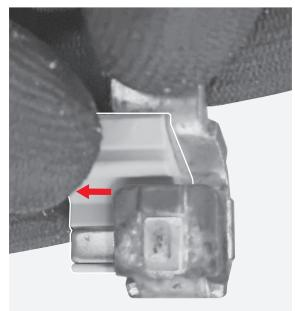
By means of the flat screwdriver remove the metal plate mounted on the the plastic part constituting the fixed contacts.
