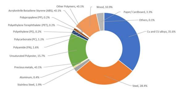
Figure 1: Composition of E6.2 6300A H - 3P IEC Withdrawable Circuit Breaker
