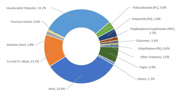
Figure 1: Composition of XT4 IEC-3P-N-S-H-L-TMA 250A
