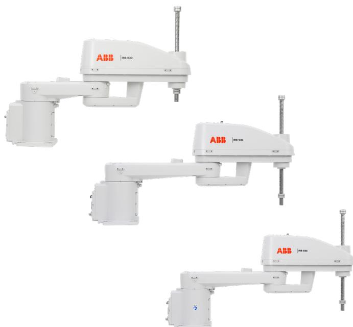
The IRB 930 is a 12-kg or 22-kg high payload SCARA robot that boosts throughput by up to 10% with class-leading speed, accuracy, internal cabling, and extraordinary downward force.
