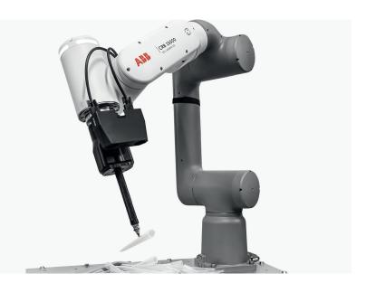
The Bin Picking Vision Function Package simplifies the robot-assisted gripping of objects thanks to integrated artificial intelligence.
