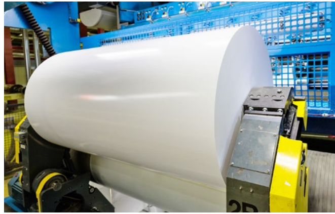
The winder at Jujo Thermal converts the parent reels coming from the paper machine into smaller rolls.
