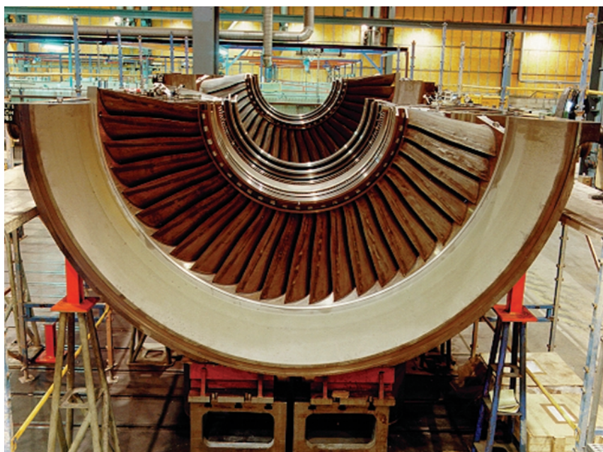
Leaned last-stage stator vanes assembled in the inner casing
