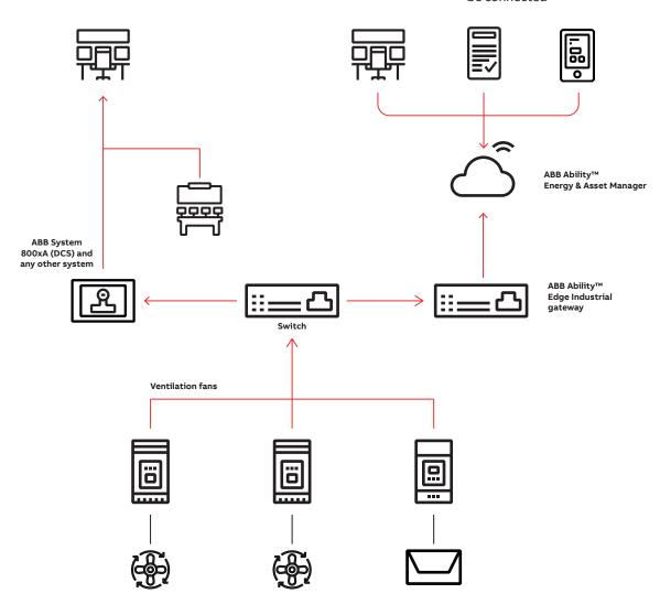
Digital offering with UMC100.3 for controlling and monitoring ventilation systems with cloud connectivity For  $0.06\,\mathrm{kW}$  to  $500\,\mathrm{kW}$  motor ratings at  $400\mathrm{V}$  AC
