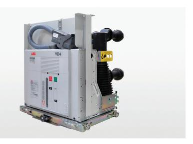
ABB offers a new IEEE 15 kV class medium voltage vacuum circuit breaker with the EL mechanism, new recyclable embedded poles up to 15 kV, 40 kA, 2000 A with 10,000 M2 Class mechanical operations, and 1200 A C2 Class back-to-back capacitive switching and out-of-phase switching test compliance.
