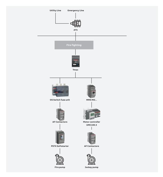
Note: Installation of a manual DOL bypass (with contactor and overload relay) for the fire and jockey pumps is recommended to provided support in the case of maintenance.
