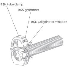
Combination with BSH tube clamp and BKE Ball joint termination
