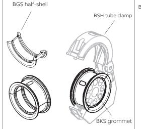
Combination with BSH tube clamp and BGS half-shells
