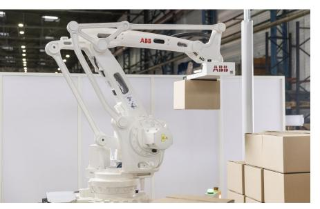
ABB's Robotic Depalletizer with machine vision enabled by proprietary ABB machine learning software combined with ABB robots. Configurations with 4- and 6-axis robots to solve a wide array of depalletizing tasks with varying box sizes, pallet patterns and heights.
