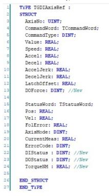
This data structure in turn contains two further data structures (*TCommandWord* and *TStatusWord*). The declarations for these are shown below:
