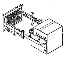
It is also possible to use: Cradle in cradle retrofit kit between Otomax circuit-breaker and New Emax + Direct replacement between New Emax and Emax 2. For any other Otomax version, only hard bus retrofill can be offered.
