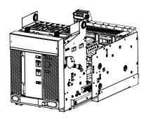
**G5:** for this size of Novomax, due to huge the dimensions, ABB has released a Cradle in Cradle retrofit kit. It consists in replacing the Novomax moving part with a special Emax 2 fixed part that fits perfectly inside the Novomax fixed part and is ready to work with a standard Emax 2 moving part. In this case, the retrofitting kit consists of:
