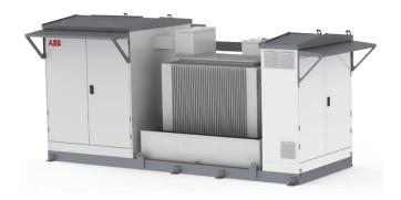
A Secondary Skid Unit (SSU) is an assembly comprising of MV switchgear, transformer and Low voltage switchboard for power collection in solar generating plants. The SSU is the power collection unit which converts the solar energy generated by the string inverters into a usable medium voltage grid voltage. The SSU is a plug-and-play solution usually installed as close as possible to the solar strings, enabling solar power to be easily and rapidly connected to the electrical grid.
