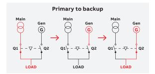
to the backup power sources. The typical delayed transition transfer sequence for the Main-Gen power supply configuration with reverse switching procedure is shown below.
