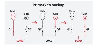
be checked. The closed transition transfer switch allows power interruption to be completely eliminated during transfers between the two available power sources. The typical closed transition transfer sequence for the Main-Gen power supply configuration is shown below.
