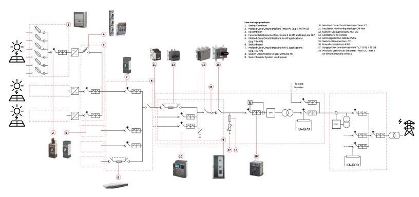
01 A typical utilityscale string inverter application and below. So, string inverters can easily be connected to standard building cabling and existing rated wiring.
