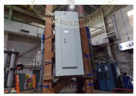
UUT wall mounted-rigid with four (4) 3/8"-16 bolts washers and lock washers. Bolts were torqued to 30 ft./lbs. Unit maintained structural integrity and remained functional per manufacturer requirement after shake table test. Contents were included in testing per operating conditions.
