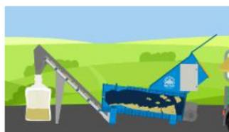
An insulation compactor takes mineral wool destined for landfill and compresses it into fine powder.
