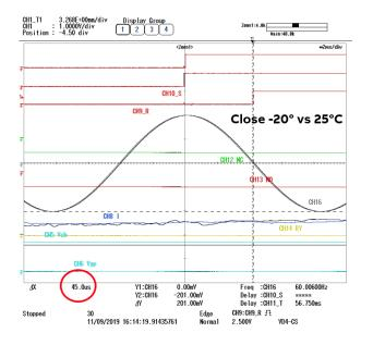
*Figure 8: Timing comparison of Close* +60°*C and* -20°*C* vs +25°*C*
