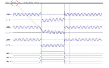
Figure 6: Making and Breaking test snapshot
