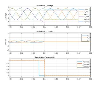
Figure 5: Open Sequence of the breaker
