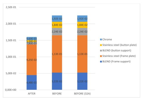
In the first graph is considered the manufacturing and use stage. As the use stage has the most impact, the rest of the stages are negligible. The product that impacts the most is the previous switch with 32A, as it is the one that consumes the most. To see the real difference made, in the second graph only the manufacturing stage is considered, which shows that there is a decrease in the impact due to a reduce in the raw material (28,93% reduce).
