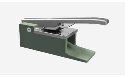
ABB's L&W Sample Cutter is used for easy and quick preparation of accurate and precise test pieces for use in tearing, bending resistance and folding strength tests, or in the L&W Autoline Elrepho Module. It is manually operated and ergonomically designed with safety features for easy and secure operation across a wide range of paper grades and grammages.
