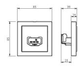
The Impressivo DCL outlet can be installed on standard wall mounting boxes (screw distance c/c 60 mm). It is safe and easy to use for the end consumer, as they can snap-in the DCL plug in the socket. The outlet is typically installed on wall but can also be installed in ceiling.
