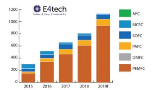
Figure 3: Annual production volumes (megawatts) for different fuel cell technologies during 2015-2019 [3]
