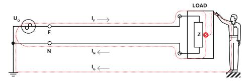
Insulation fault and current path
