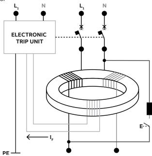
The "electromechanical" version gets around the aforementioned situation through the use of a magnetic relay, thereby ensuring stable and autonomous measurement. The DS301C, DS201, DS202C and DS203NC range falls into this category.
