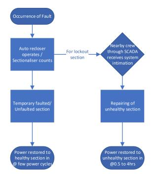
Figure 4 Power restoration with FDIR
