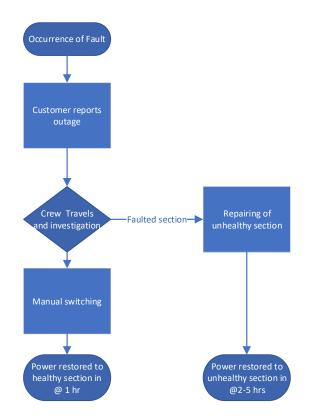
Figure 3 Power restoration without FDIR
