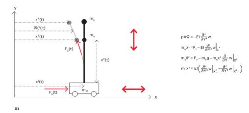
depends on the lifted load, which varies with the magnitude and position. To circumvent the damaging consequences of oscillations, the crane's operating system requires a few seconds to stabilize so that vibrations can cease before movement can continue. This process is timeconsuming and as such reduces throughput and performance.
