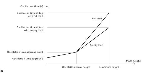
for storing and obtaining the needed system parameters ie, damping ratio and swing time.
