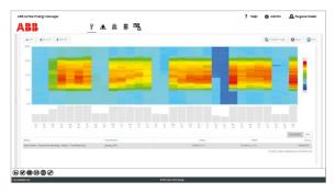
Colour block indicates energy consumption during working hours. Dark blue indicates what the out of hours or base load energy consumption should be which was part of a test completed by Enterprise Ireland to highlight that their base load was too high as indicated by the light blue.
