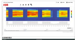
This is the profile of the building for the month after the correction of the integration issue between the BMS and the VRV air conditioning system.
