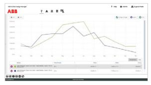
The time period comparison shows a drop in energy consumption of 17% from 2011 to 2012 which is due to more efficient operation of the AHU during store operating hours.
