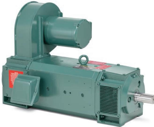
RPM III DC Motors feature a laminated square frame design which provides more power, reliability and serviceability in a smaller package. The field proven laminated frame improves commutation and heat dissipation, and requires less mounting space than conventional designs. Choose from the complete line of enclosures including:
