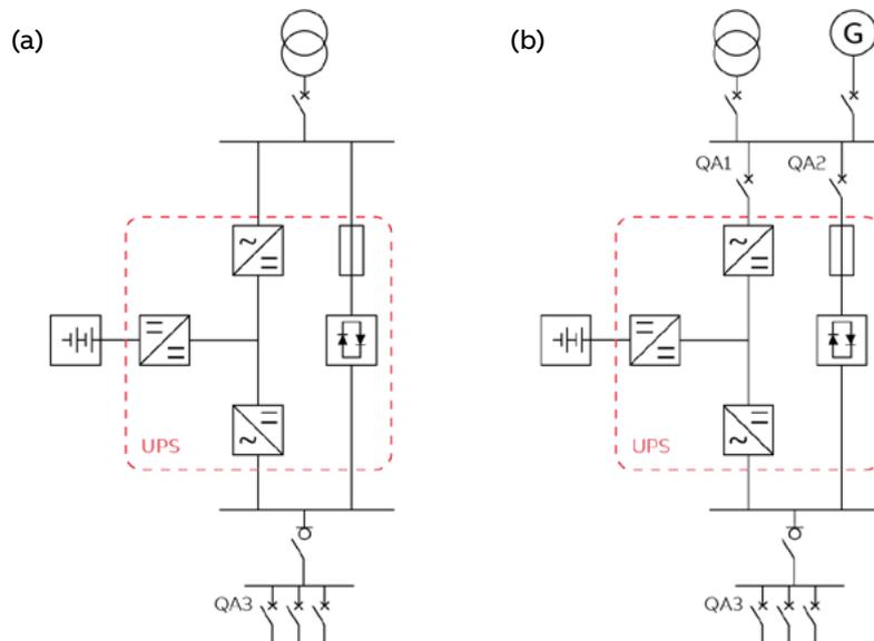
In **case of a fault condition at the load side downstream**, the UPS will rapidly **switch** from double conversion operating mode **to static bypass**, made of a thyristor bridge and a fuse or a thyristor bridge only, depending on the UPS model. The **selectivity** to be considered is the one **between the downstream circuit breaker and the fuse in the static bypass**.
