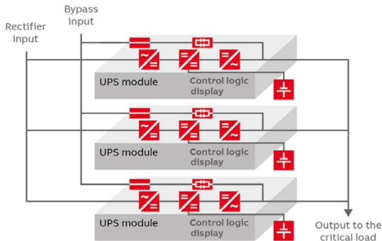
Coming back to selectivity, because the fuse inside every UPS module is considered in parallel with the other, two different co-ordinations need to be verified:
