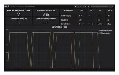
A dashboard view of Winder Performance Optimization showing how it can help improve production capacity
