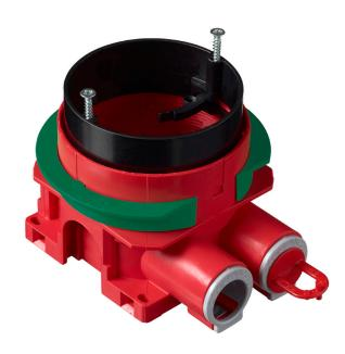
Installation box is certified to be used in El60 and El30 fire rated walls with different thicknesses due to its adapter ring. The AU60.10FR contains a fire cushion, made of expanding material, that prevents fire from spreading to walls.
