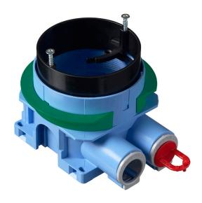
The universal hollow wall box AU60.10 is suitable for 1-2-3 layers of gypsum boards, and all other wall structures with wall thickness 12,5-40 mm without accessories. Box includes a rotating, steplessly adjustable installation ring with proven functionality. Can be mounted with box support and with truss fixtures.
