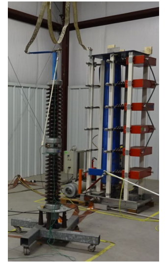
Existing ABB impulse tester, having to “raise the roof” for new tester
