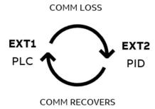
To allow the PID loop controller to work during the communication loss, the PID controller needs to be fully commissioned. You need to wire the analog feedback signal from the actual process to AI2 (remember, this feature is needed only when the communication is lost thus you cannot use the feedback over fieldbus) and you need to set the setpoint source as either constant, control panel or via analog input (normally AI1) as well. The settings may be adjusted very easily via the Primary settings.
