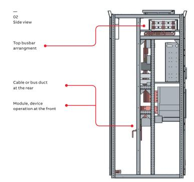
Full interchangeability of modules between different MNS designs for front or rear access.
