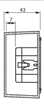
The surface mounting boxes are spacious enough for installing ABB dimmers and other high electronic components.
