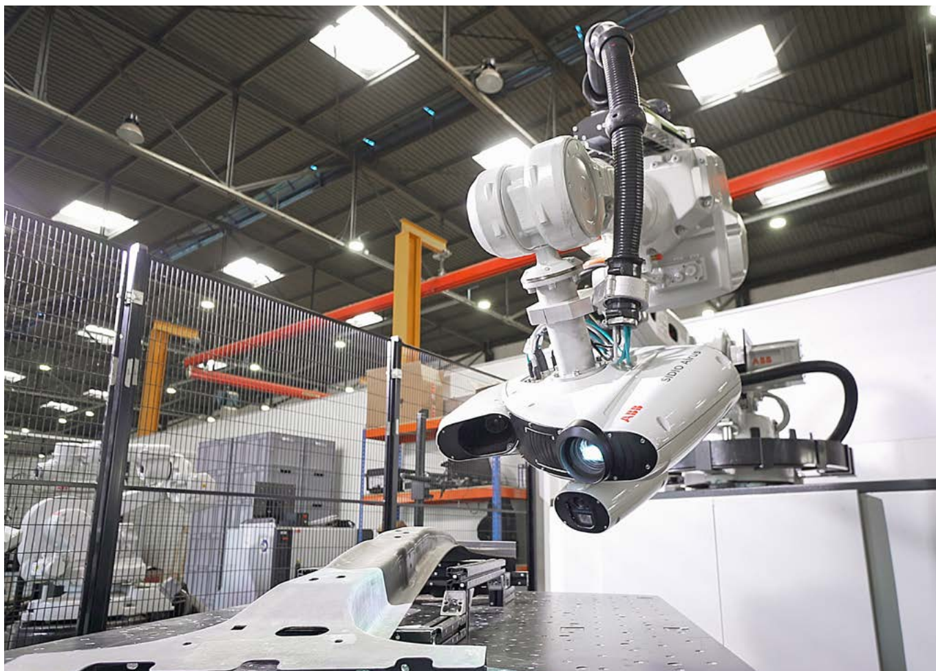
Robotic 3D quality inspection is one example of a technology originally developed for the automotive industry that can be applied to help improve quality and productivity in construction applications.
