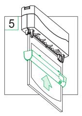
Re-attach the signplate cover by sliding it over the signplate. Make sure that it is orientated correctly
