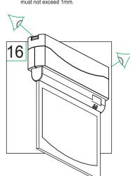
Ensure that the clips on the main body fully engage into the first fix by making a visual inspection.
