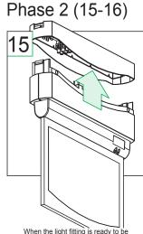
When the light fitting is ready to be commissioned, simply push the main body into the first fix. Make sure that
