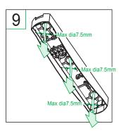
Pull the cable through into the first fix. The cable diameter must not exceed 7.5mm. You may not need to use all of the cable entries
