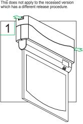
To release the light fitting from the first fix, simply push in the clips at
