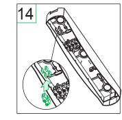
There is a facility for a single terminal block (not supplied) if earth continuity is required.
