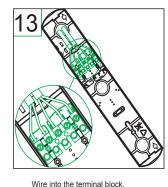
P=unswitched live P1=switched live N=Neutral +=Rest mode positiive (if required) -=Rest mode negative (if required)
