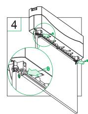
It is optional to fit the signplate securing screws. However, we recommend that they are fitted in environments where the signplate may suffer impact.
