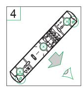
Line up the first fix cable entry hole(s) with the cable in the mounting surface Make sure that the arrows are facing
