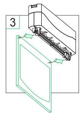
Remove the signplate from the packaging. Making sure that the signplate is facing in the correct direction, align the holes over the lugs indicated
