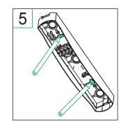
Mark through the slots onto the mounting surface and remove the first fix.
