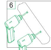
Drill the holes in the mounting surface to accept the fixing screws (not supplied). Use wall fixing hole plugs if required.
