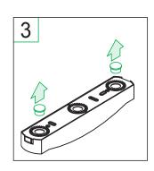
Remove the hole plugs to coincide with the intended cable entry position. Replace the hole plug(s) in the hole(s) which will not be used.
