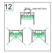
The maximum diameter cable to go under the terminal block is 7.5mm Cable(s) must not pass over the terminal block. The terminal block
