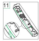
Make sure that the cable wires go below the indication mark, otherwise the finished product will not fit together properly.
