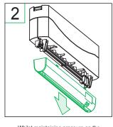
Whilst maintaining pressure on the signplate cover, pull it away from the light fitting.
