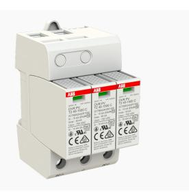
Type 2 SPDs for photovoltaic applications are capable of discharging the lightning currents within an electrical system resulting from indirect lightning events. They have effective voltage protection ratings keeping damaging voltage peaks from exceeding the withstand voltages of the protected equipment.
