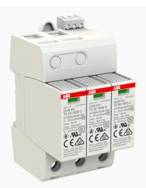
Type 2 SPDs for Photovoltaic applications are capable of discharging the lightning currents within an electrical system resulting from indirect lightning events. They have effective voltage protection ratings keeping damaging voltage peaks from exceeding the withstand voltages of the protected equipment.
