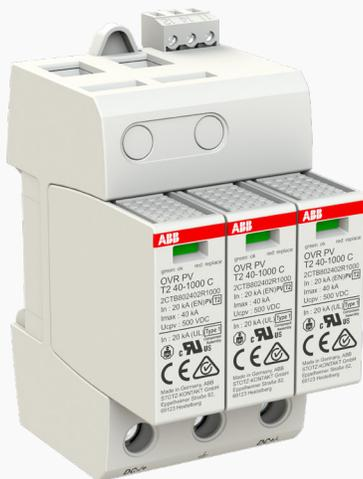
Type 2 SPDs for Photovoltaic applications are capable of discharging the lightning currents within an electrical system resulting from indirect lightning events. They have effective voltage protection ratings keeping damaging voltage peaks from exceeding the withstand voltages of the protected equipment.
