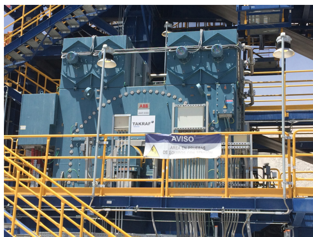
Figure 3. ABB GCDs are robust, require minimal maintenance, and can boost the energy efficiency of high-power systems by 2 – 3%.
