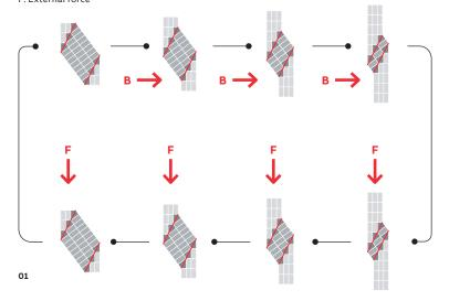
01 Applying an external magnetic field (B) leads to a proportional deflection of the folded crystal structure. In standard applications, resetting to the original shape is done via an external force (F).
