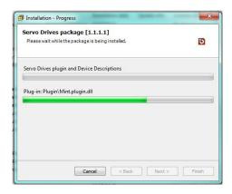
Once installed Automation Builder will be restarted automatically for the installation to take effect. Once restarted you can now re-open your original Automation Builder project and when adding objects to the EtherCAT master device you will now see the latest list of servo drives that can be added to the device tree. Click on the appropriate Mint servo drive package object to add it to the device tree...
