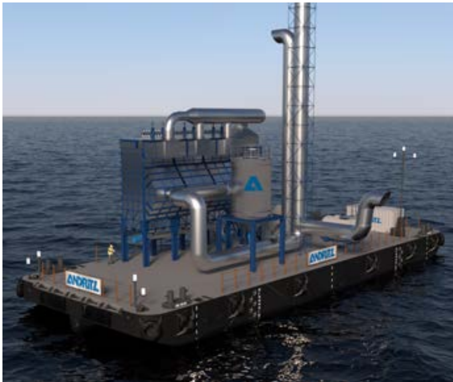
Andritz port barge design for vessels not fitted with a scrubber
