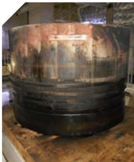
Piston with scuffing and deposits clearly seen (©Chevron)
