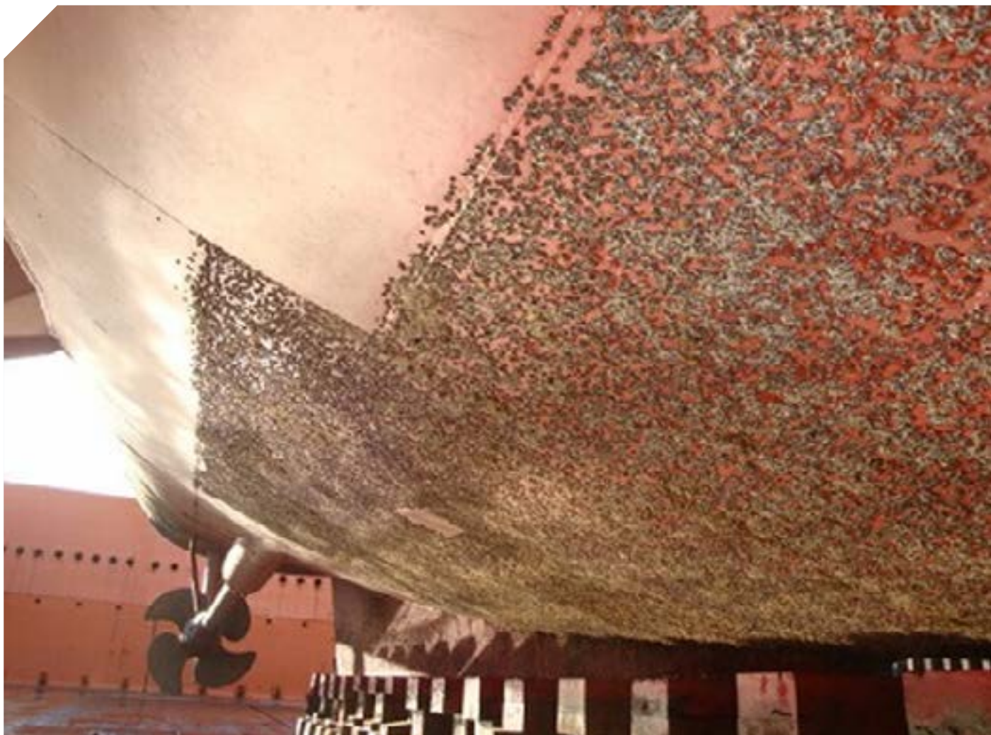
Underwater areas of a ship's hull can get badly fouled (credit: I-Tech)
