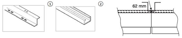
The Z-profiles are bolted together by means of 2 C-profiles ② and sliding nuts + M8 bolts ③ for fixation. The VMS boxes can be mounted directly on the front of the Z-profiles by means of M5 x 16 Torx screws ④. The Z-profiles can be mounted on the floor using the stand supports ⑤ + ⑥.
