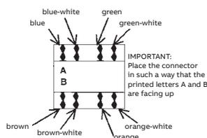
2b Wiring according to T568B:
