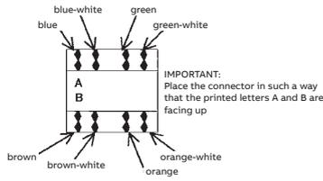
2b Wiring according to T568B:
