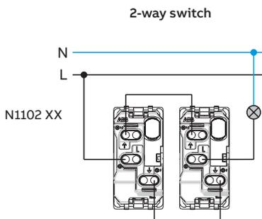
2-way switch - Intermediate switch - 2-way switch
