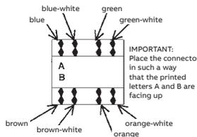
2b.- Wiring according to T568B:
