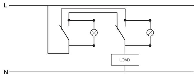
The two warning lights switch on and off respectively when the load is in the OFF and ON state.
