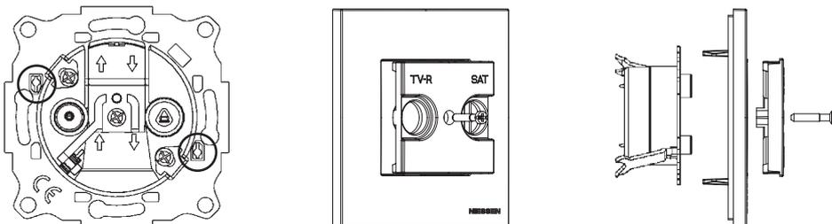
2. There are two options of mounting the cover plates: a) cut the clamps that are facing the small holes.
