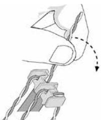
2.5 Insert the end piece into the module.
