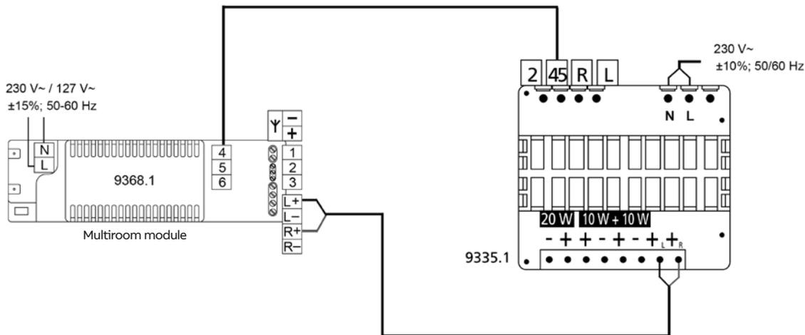
Wiring diagram for 9329.1 loudspeakers to 9335.1 sound amplifier
