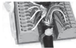
**Note:** Using a strap for fixing the cable to the board it is recommended to avoid disconnections. For this the plates have two through-holes at its rear end.
