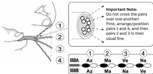
2.2.- Position each of the four pairs in the holes of the end piece.
