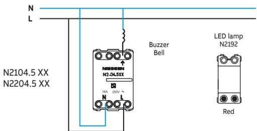
Push-button for relay with locator lamp
