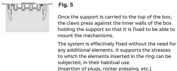
Insertion of a 1-module mechanism in a mountin plate with elastic claws.
