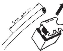
2 Bring the cable close to the connector, with the jacket at approx. 6 mm from the connector. Insert the cables into the corresponding slots as indicated by the cable color-wiring configuration for T568A or T568 B (as shown in Figures 2A and 2B).
