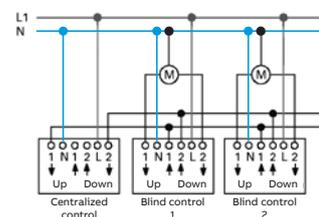
The IR button 8439.XX and the programmer 8165.3 can control a group of blind motors by operating the auxiliary inputs ("1" and "2") of the blind control device. Using a two-pole switch for blinds, the group of blinds can be moved manually or the sensor can be activated for periods of absence. The recessed device 8161.2 is used to control:
