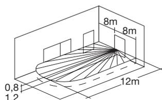
In these applications, the light sources must be outside the detection area to prevent the disconnection due to a Sensor Switch being interpreted as a thermal variation by the other Sensor Switch, causing an unwanted connection.
