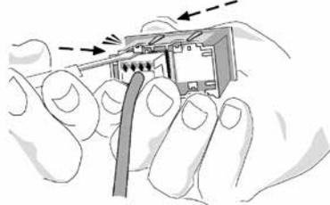
5.2 Pry upwards to release the upper hook.
