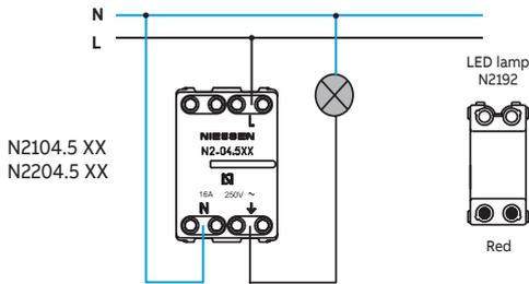
Push-button for buzzer / bell with locator lamp
