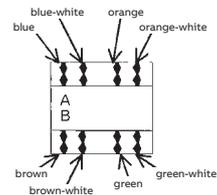
3.- Push the cables against the end of the slot and cut them flush to the connector. Use an IBDN 110, BIX, KRONE wiring tool, or a similar type 110 tool.
