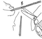
1.5.- Cut the mesh (if it has one) and the cord at the same level of the jacket.
