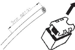
2.- Remove the back cap from the connector. Strip approx. 5cm off the jacket and discard the cable cutter cord.
