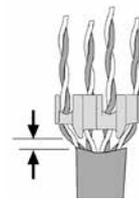
2.4 Place the pairs in the direction of the end piece slots.
