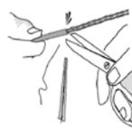
1.4 Cut the mesh (if it has one and the cord at the same level of the jacket).
