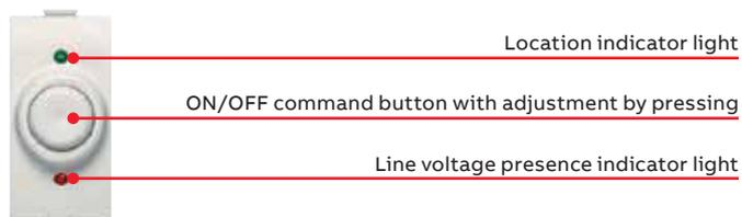
Electronic dimmer with pushbutton control for resistive and inductive loads 60-500W 60-500VA 230V~ -50/60Hz (visible in the dark).
