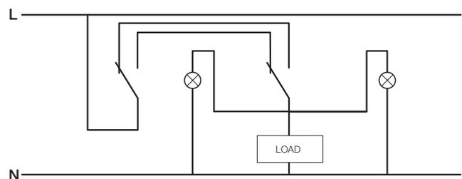
Two warning lights placed in parallel with the load (they switch on and off with it).
