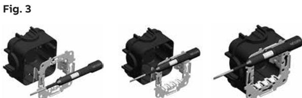
The assembly is pressed into the housing.
