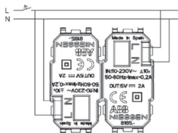
3.3.- Fig. 5.- Installation of USB charger with two outlets 8185.3
