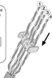
2.3 Ensure the end piece is located as close as possible to the edge of the jacket.
