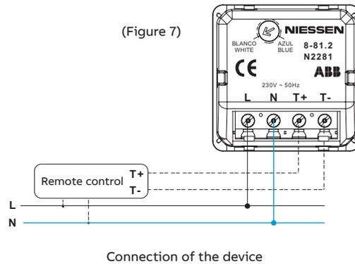
\* The voltage of the remote controls may be 9, 13 or 24 Vdc.
