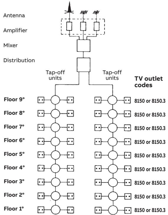
In this diagram all final outlets are the same. References 8150 or 8150.3 can be used equally.
