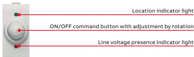
Electronic dimmer with rotary control for resistive loads 100-500W 230V~ 50/60Hz (visible in the dark).
