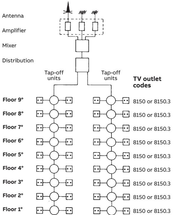
In this diagram all final outlets are the same. References 8150 or 8150.3 can be used equally.
