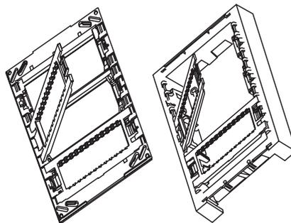
3. The mechanisms are inserted in the mounting plate by pressure.
