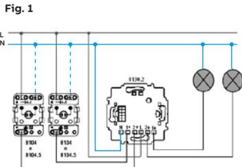
8130.2 with auxiliary buttons (8144.2, 8104.5) and two lamps.
